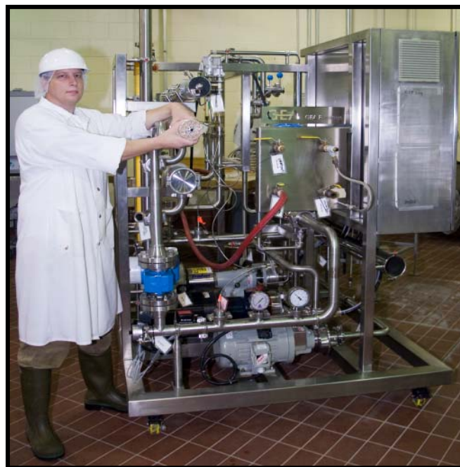
Figure 1: The pilot plant membrane filtration system (GEA Model R) is a flexible unit able to perform pilot plant studies on the full range of membrane filtration technologies under a wide range of operating conditions.
